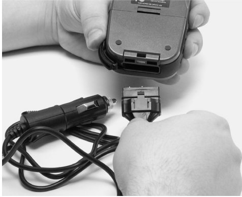
Attach external power cable to iFINDER.
