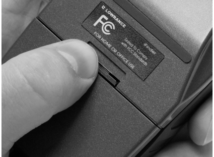
Replace battery compartment cover. Align tabs with slots in the base, left. Press latch firmly until it clicks, as shown right
